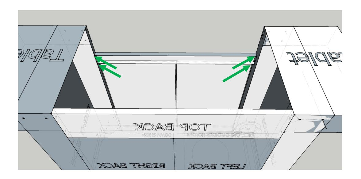
10 FIRE WALL: Fix the fire wallwith the 2 M4 nuts
