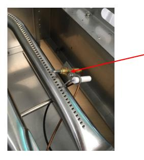
1- Brush and clean the thermocouple on burner
