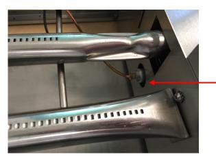
2- check that the screw is correctly tightened
